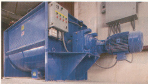
PVC and wood fibers for extruded products are mixed in this Munson paddle blender. PVC is loaded into the blender from the plant's main PVC feed line (the horizontal gray pipe located near the ceiling to the left of the blender). Mixed material is discharged from the bottom of the blender and loaded into a moveable hopper by an auger (the long, white pipe in the foreground).
