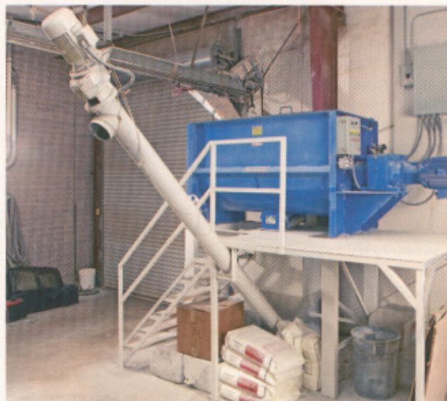
A closeup of the paddle blender, showing the control panel and the machine's 10-hp motor.
